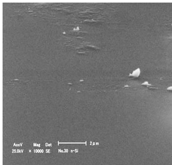
Figure 3 The scanning electron micrograph (SEM) topography image of typical as-grown (25°C) a-C:N film on silicon substrates. (Magnification: \times 10 K).
